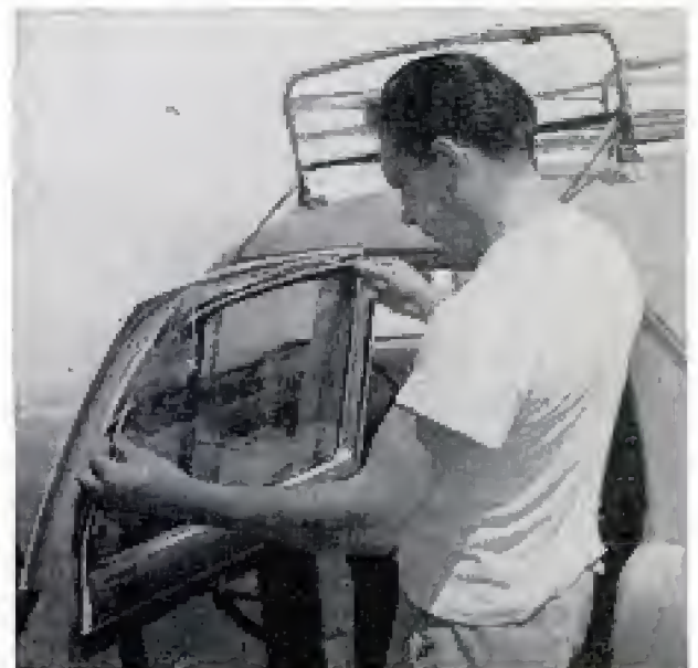
As window frame is replaced, screen is stretched and made smooth. Window still can be opened and closed
